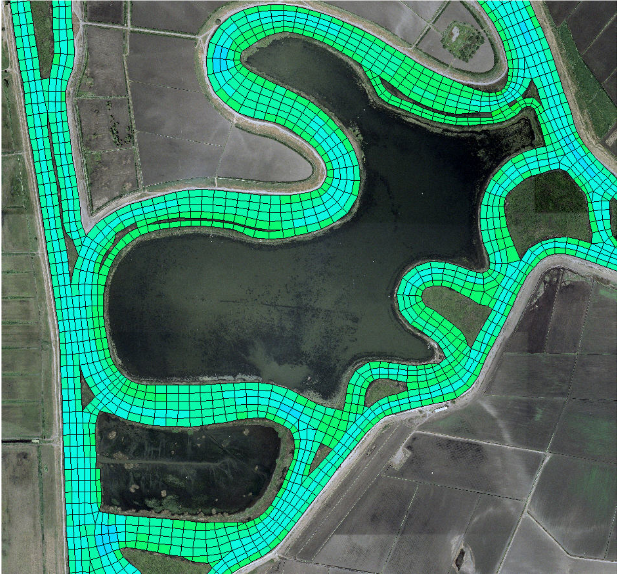
Figure 6.2-3 Location of several islands south of Franks Tract, including Little Mandeville Island (center) and Rhode Island (lower left), which flood on high tides or are permanently flooded, but are not included in available Delta bathymetry or the current model grid.
