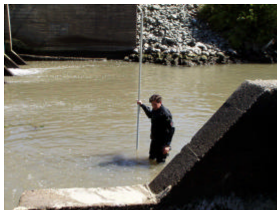
Figure 11. Evaluating the downstream apron
