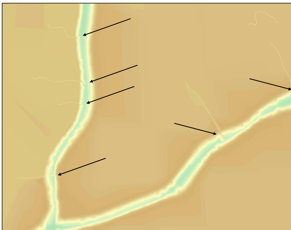
Figure 11-5 Historical DEM artifact example: artificial groins caused by interpolation near junctions. Grid is shown near Sacramento – Cache Slough confluence.
