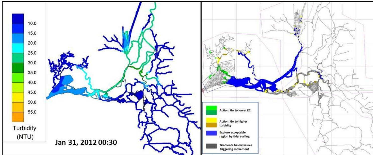
Figure 29 Turbidity contours and particle location in the RMA model grid on Jan. 31, 2012.
