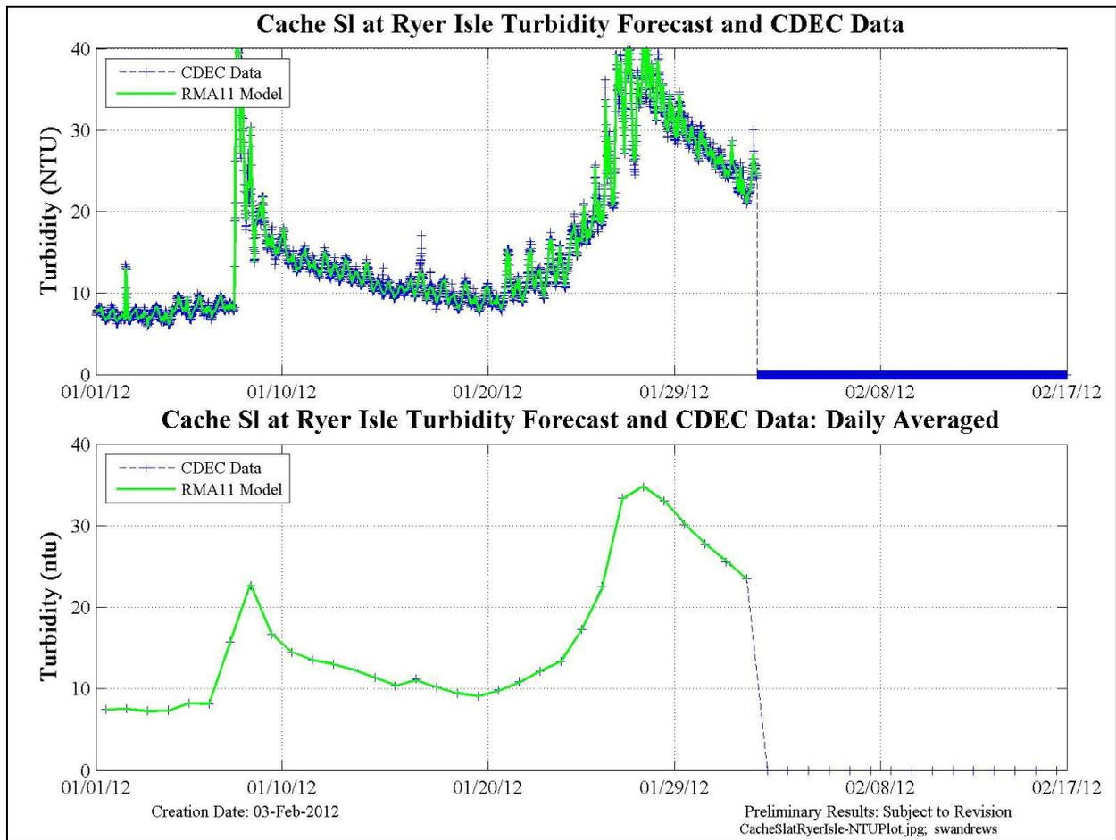
**Figure 8** The Cache Slough at Ryer Island internal turbidity BC was compiled from CDEC data. The boundary condition was not applied beyond the end time of the observed data. Zero values indicate the end of data application period (blue).
