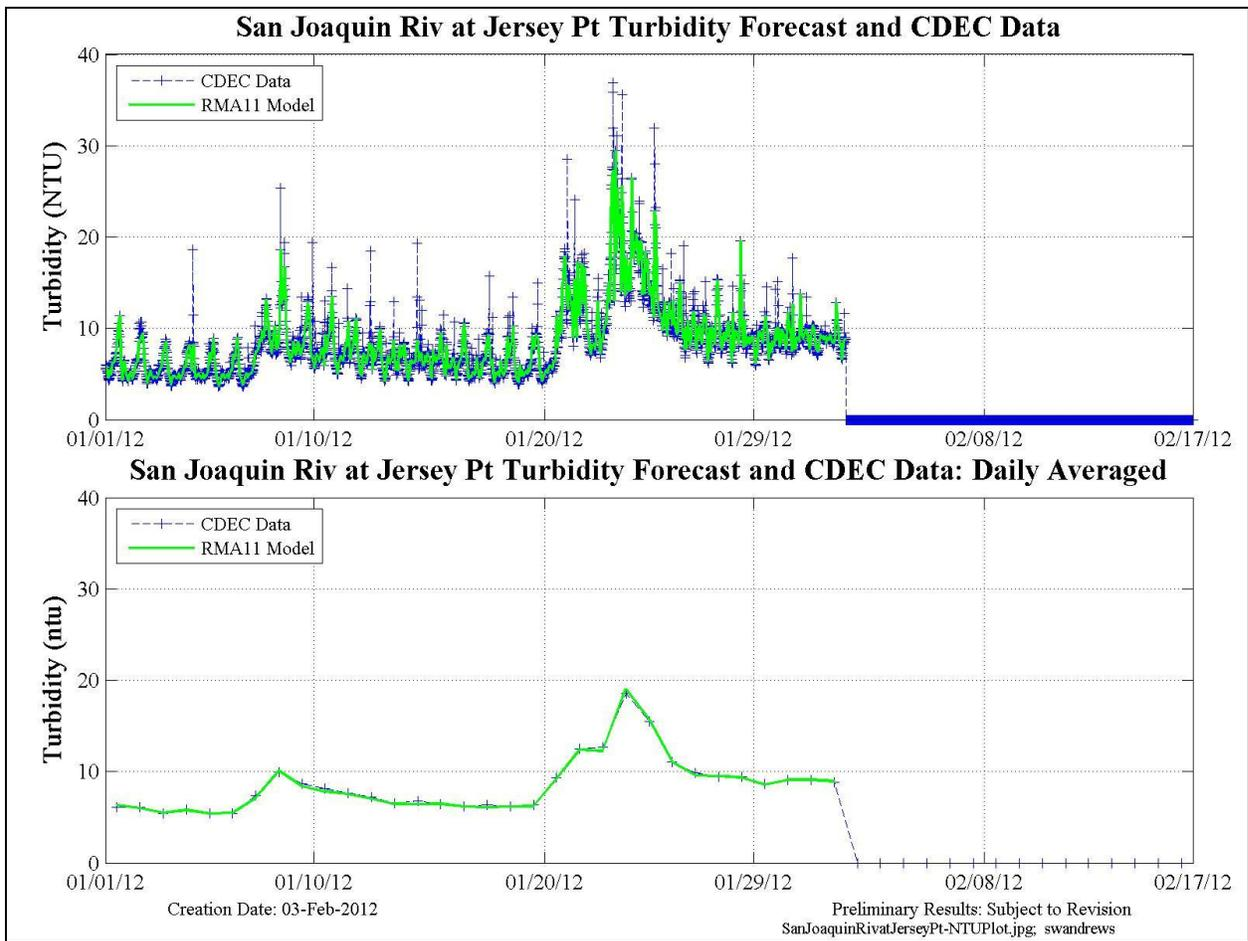
**Figure 11 The San Joaquin River at Jersey Point internal turbidity BC was compiled from CDEC data. The boundary condition was not applied beyond the end time of the observed data. Zero values indicate the end of data application period (blue).**
