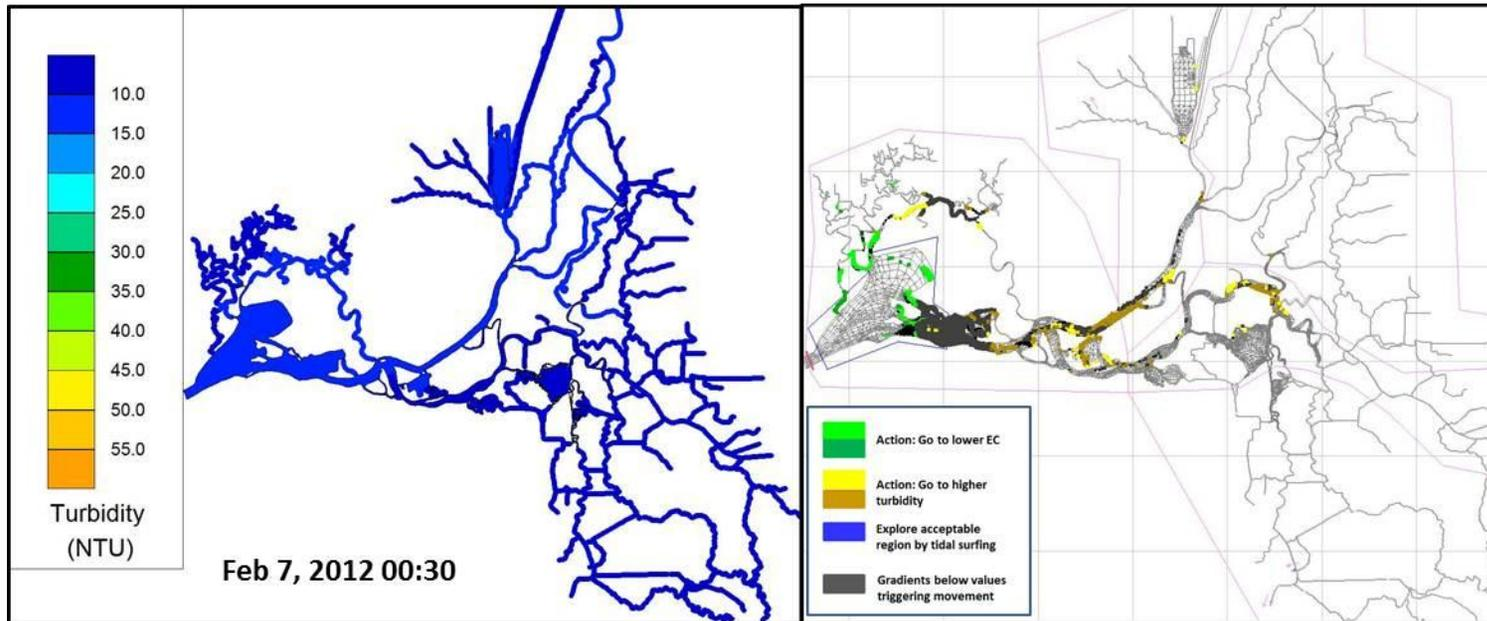
Figure 30 Turbidity contours and particle location in the RMA model grid on Feb. 7, 2012.
