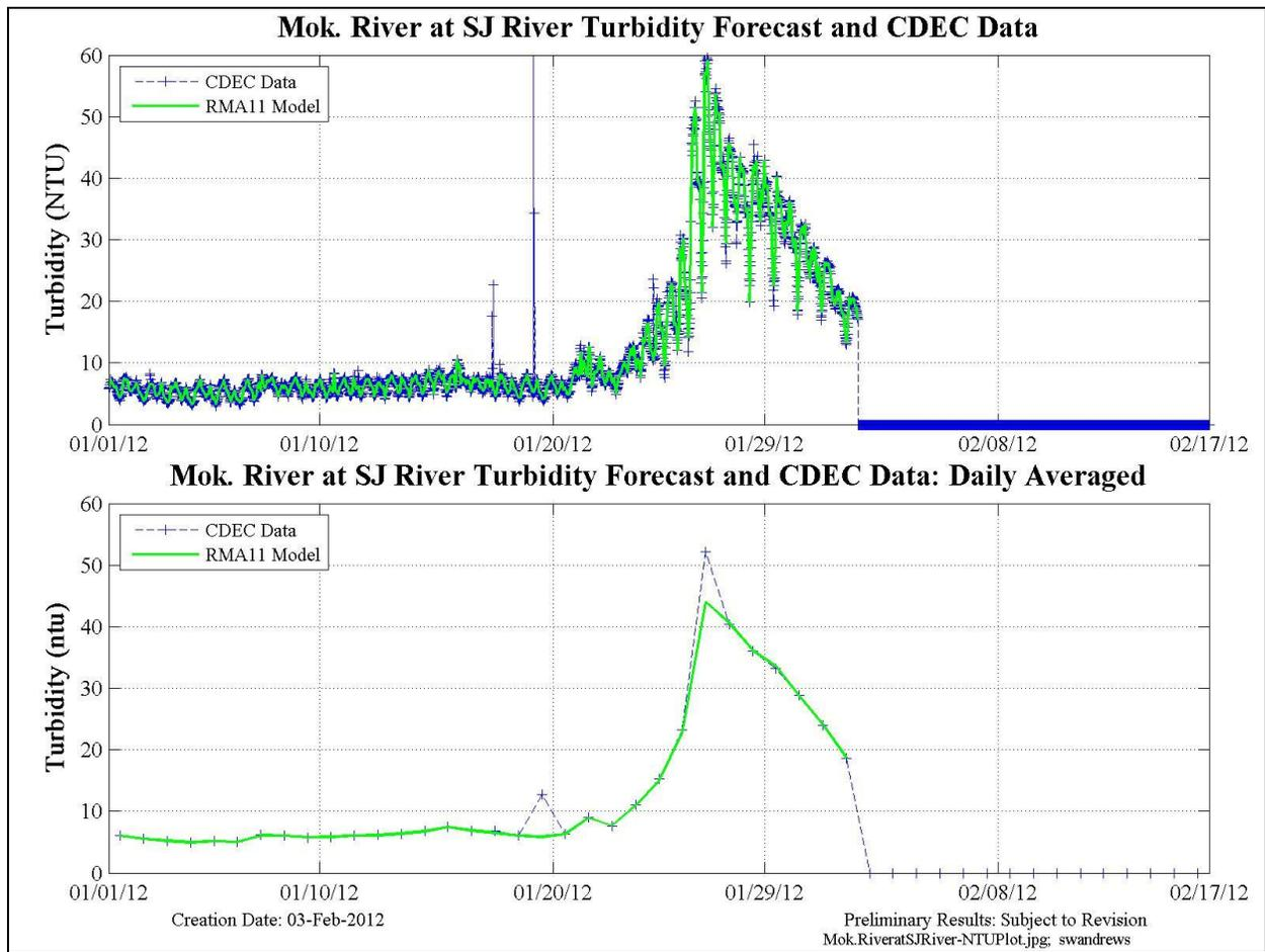
**Figure 9** The Mokelumne River at the San Joaquin River confluence internal turbidity BC was compiled from CDEC data. The boundary condition was not applied beyond the end time of the observed data. Zero values indicate the end of data application period (blue).
