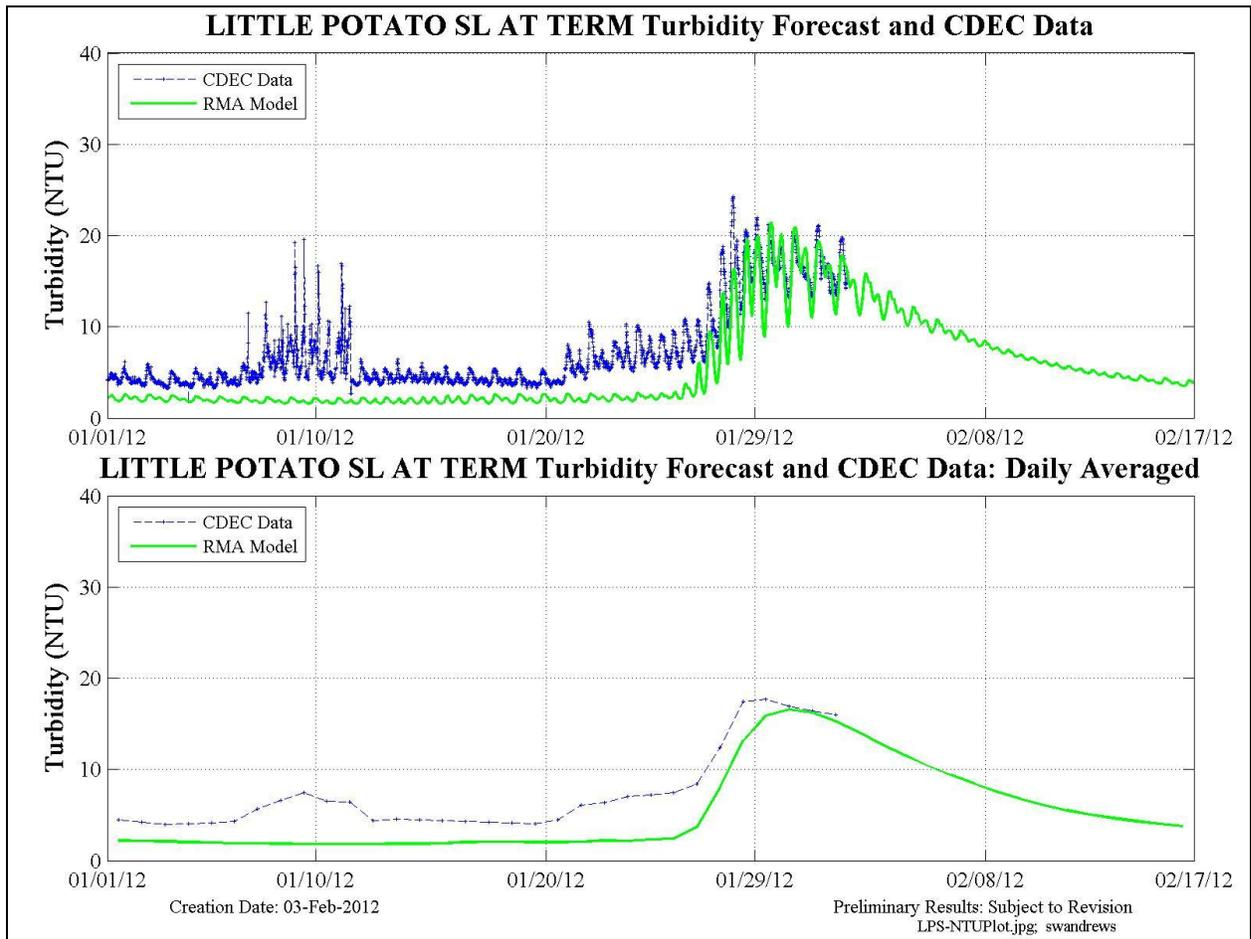
**Figure 23 Model forecast and raw CDEC data at Little Potato Slough at Terminus. Both 15-min (upper) and daily averaged (lower) plots are shown.**
