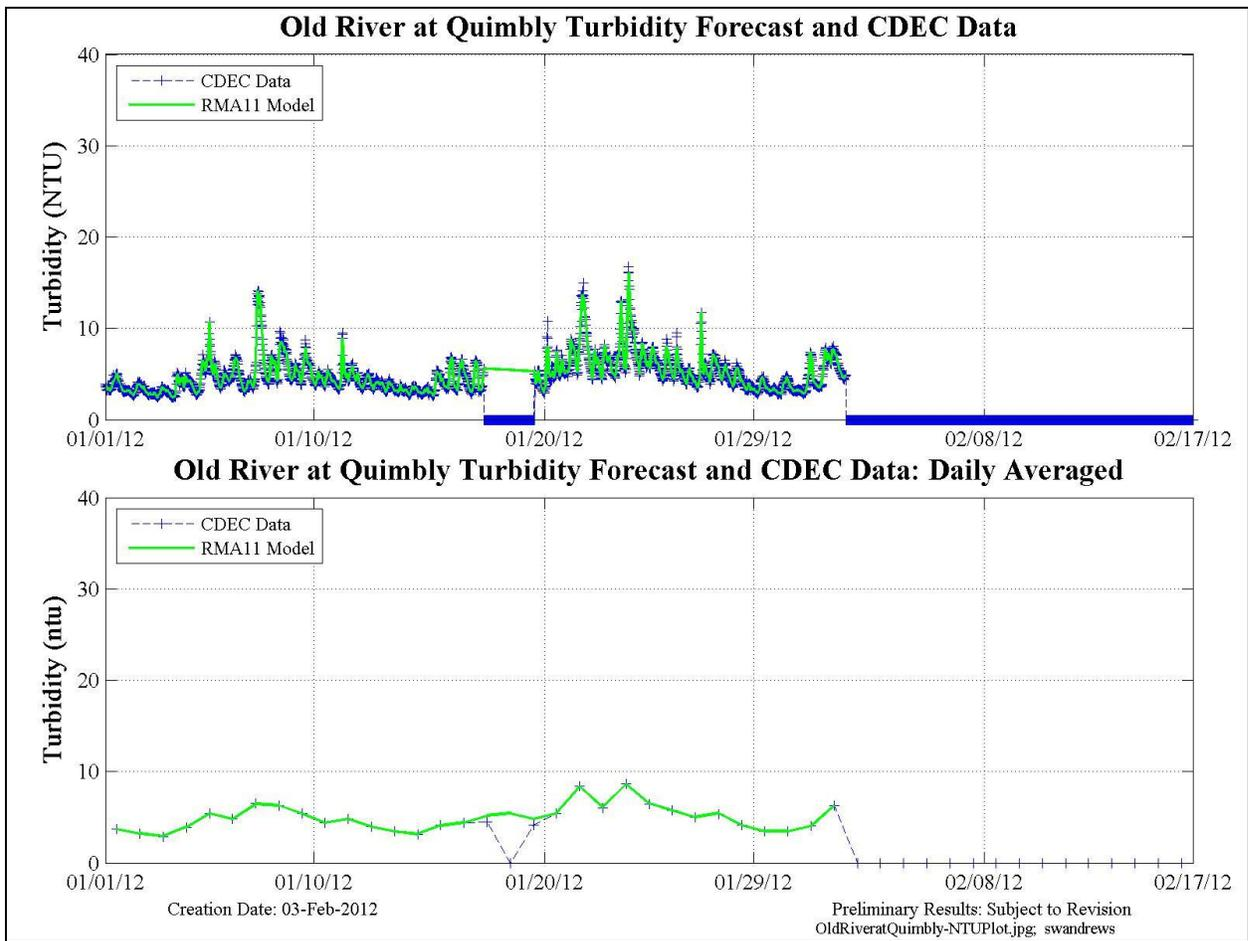
**Figure 10** The Old River at Quimby Island internal turbidity BC was compiled from CDEC data. The boundary condition was not applied beyond the end time of the observed data. Zero values indicate the end of data application period (blue).
