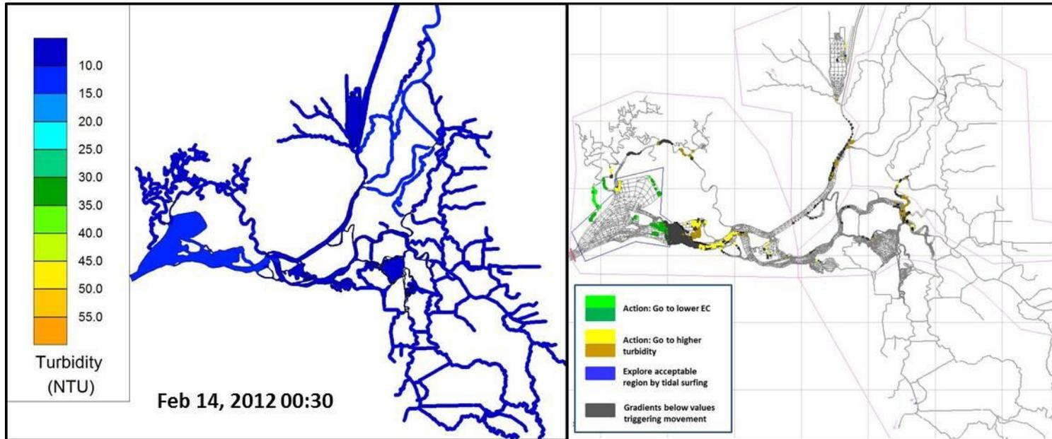
Figure 31 Turbidity contours and particle location in the RMA model grid on Feb. 14, 2012.
