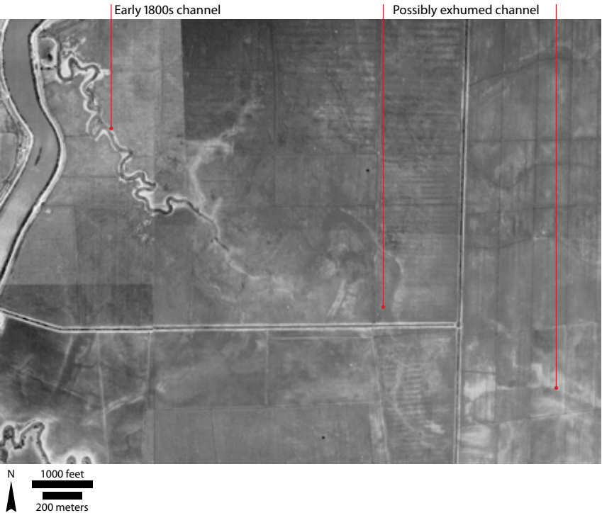
Figure 2.8. A recently active (pre-reclamation) channel that is a high interpretation certainty level channel can be seen (upper left). The fainter, wider, and less sinuous channel signature in the lower right that joins the channel may not have been active in recent history and may be an older channel whose inorganic soils were exposed in the process of reclamation as the overlying peat was oxidized (Atwater pers. comm.). (USDA 1937-1939)
